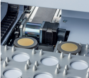
Flexible sample feeding: Automated loading via conveyor belt and manual loading with optional priority mode.
