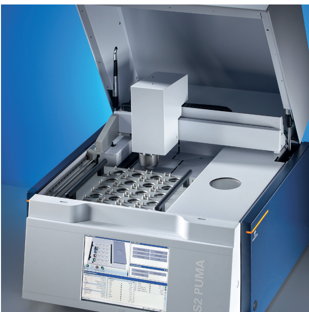
The XY Autochanger for high throughput
