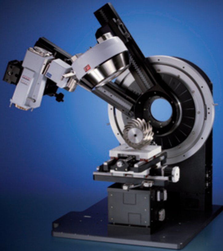
Residual stress setup with vertical goniometer, UMC stage and VANTEC-500
